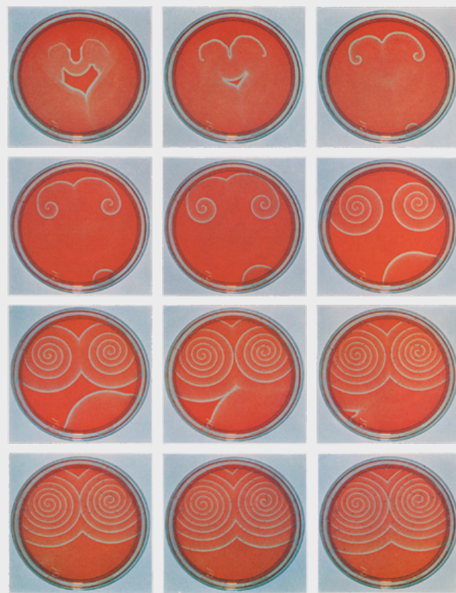
1974, Spiral Reaction: "Spirals of chemical activity form in a shallow dish of red reagent. A blue ring was induced by touching the surface of the solution with a hot filament, then the dish was rocked to break the ring. The free ends of the fragmented circular wave each curl around a pivot point, winding up into spirals." Photographs were taken over eight minutes.
