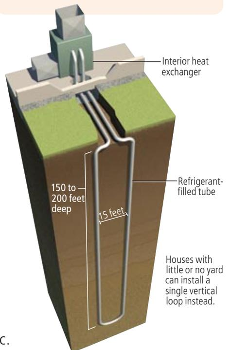
Houses with little or no yard can install a single vertical loop instead.
