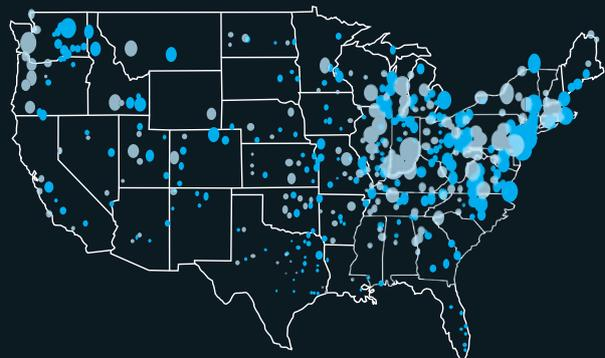
The entire East Coast and much of the rest of the country would lose power. This map shows the blacked-out regions expected from a severe storm like that of 1921, which would induce ground fields of about 20 volts per kilometer. Scientists have yet to model the effects of a full-blown 1859-like storm on the power grid.
