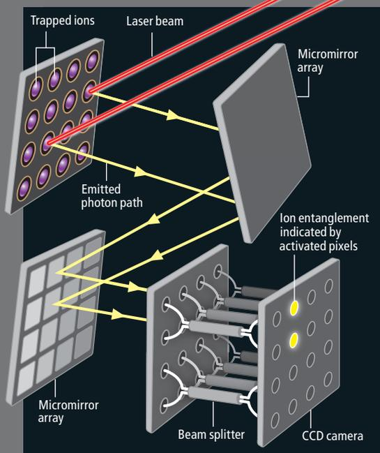
by repeating the process and simply waiting for photons to be simultaneously counted on the detectors. Once this occurs, even though the ions may be widely separated, the manipulation of one of the qubits will affect the other, allowing the construction of a CNOT logic gate.
