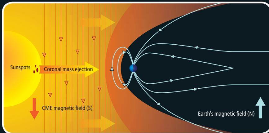
**MAGNETIC RECONNECTION:** The solar gas has its own magnetic field, and as it streams past our planet, it stirs up turbulence in Earth's magnetic field. If this field points in the opposite direction as Earth's, the two can link up, or reconnect—releasing magnetic energy that accelerates particles and thereby creates bright auroras and powerful electric currents.
