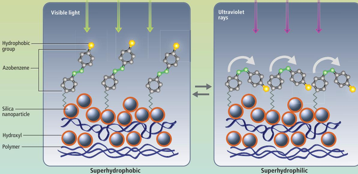
▲ Researchers at Pohang University of Science and Technology in South Korea attached a molecule based on azobenzene on top of polymer-silica multilayers [see box on preceding page]. A hydrophobic group on the end of the molecule, along with the roughness of the layers, makes the surface superhydrophobic (left). In ultraviolet light, however, the molecule bends, burying the hydrophobic group and making the surface superhydrophilic (right). Visible light promptly restores the original condition.
