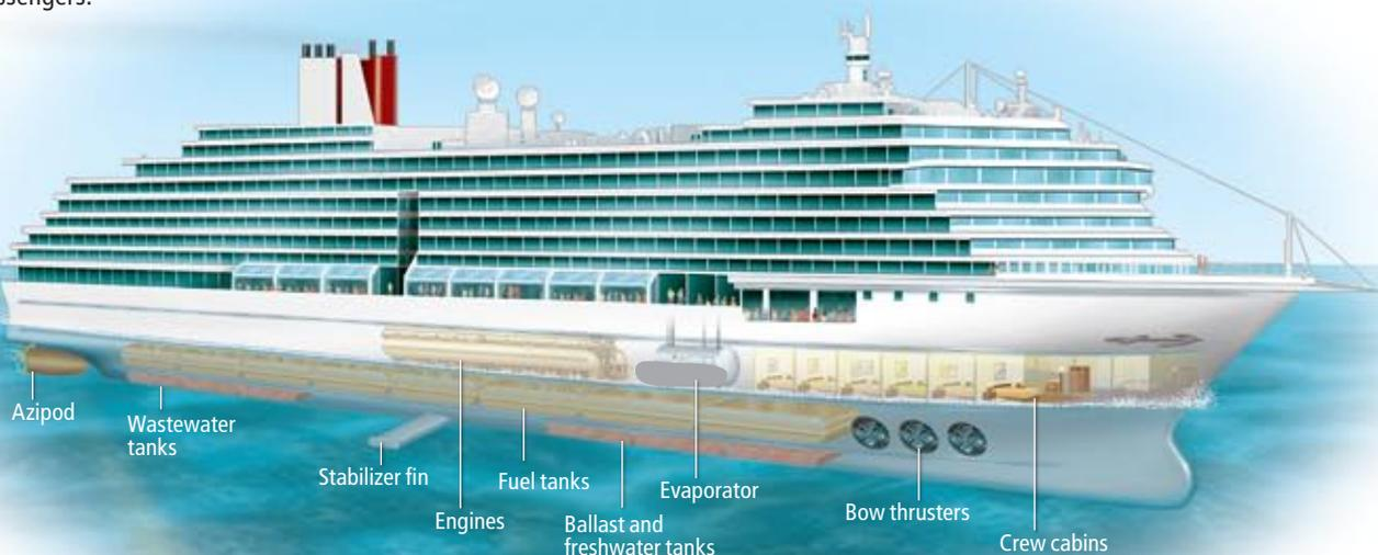
→ **TWO STEEL FINs**, 24 feet long, counteract starboard and port rolls (*shown*) caused by ocean swells.
