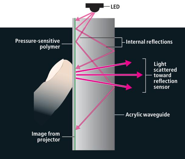
To create a signal, LEDs bounce light through the acrylic sheet. No light escapes. But if a finger is placed against the face (above), light will scatter off it toward the sensors. Also, a pressure-sensitive coating flexes when pressed firmly or lightly, making the scattered fingertip signal appear slightly brighter or dimmer, which the computer interprets as more or less pressure.
