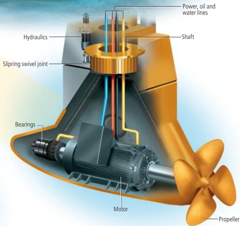
→ **PROPELLER** is turned by an electric motor inside the Azipod, which draws current from generators powered by the ship's engines. Hydraulics can swivel the unit 360 degrees. Motor current, lubricants and cooling water pass through the swivel joint.
