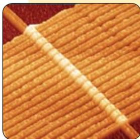
**MEMRISTORS, 17 in all, were made with 50-nanometer-wide platinum wires crossed by another wire.**
