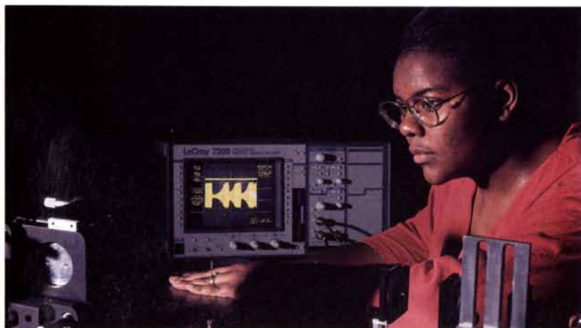
INTENSITY OF LASER , shown on oscilloscope screen as chaotic bursts over time, is monitored by Georgia Institute of Technology graduate student Zelda Gills. Photo: Margaret Barrett, Georgia Institute of Technology.
