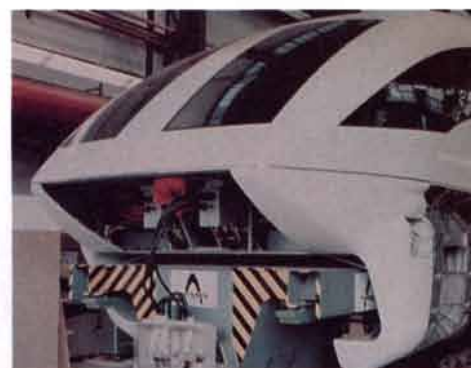
TRANSRAPID 07, the German maglev that is being readied for commercial service, is built with nonsuperconducting magnets attached to the vehicle. These magnets are attracted upward to within an inch of a steel rail on the guideway.
