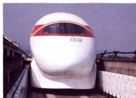
MLU002, a Japanese maglev prototype destroyed in a fire last year, has superconducting magnets that interact with metal coils in the guideway's side walls. Magnetic fields induced in the coils create a repelling force that lifts and stabilizes the vehicle four inches above the guideway.
