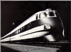
The Pendolino: The Fiat-built train sports a bar, a first-class galley, and a phone booth. Its big reason, though, is the ability to lean into curves at speeds of up to 250 kilometers per hour.
