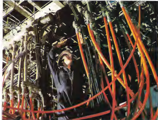
Rectangular MHD channel generates power via a high-voltage switching room (see photos on opening pages). From there, current travels to resistance loads (far left) or into a power grid. Hot gases from the channel rush on to equipment (above) that slows and cools exhaust before it's vented through a smokestack. (In full-scale operation, heat in the gas would be used to generate steam and drive electrical power.) Engineers monitor charts to assess how well experimental gear performs (left). High-tech plant relies on old-fashioned fuel: coal. But the futuristic MHD process is far more efficient than traditional burners or nuclear plants.
