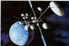
Geostationary platforms, sprouting sets of antennas, would help reduce congestion in space.
