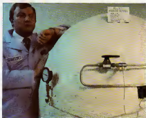
Billings attends to one of his hydride tanks, able to hold 60 pounds of hydrogen.
