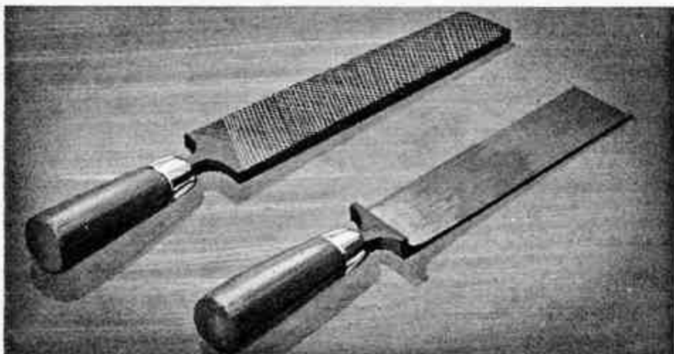
SCRAPER MADE FROM FILE
